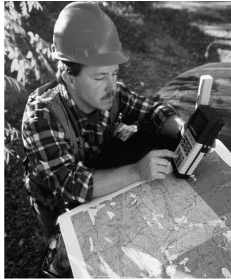
A forester uses a global positioning system (GPS) to accurately pinpoint his location within an undeveloped landscape. Using satellite technology, a GPS can not only determine latitude and longitude, but also heights above sea level. Stone/Getty Images.
