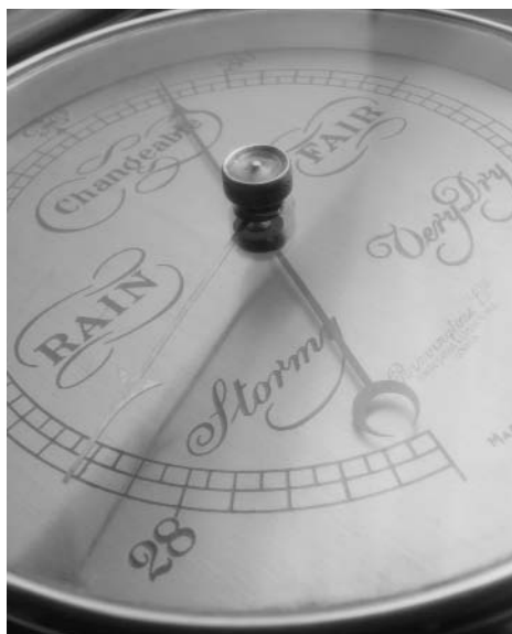
A barometer is a type of gauge that measures atmospheric pressure, which makes it useful in detecting high and low pressure systems that can predict changes in the weather. Taxi/Getty Images.
