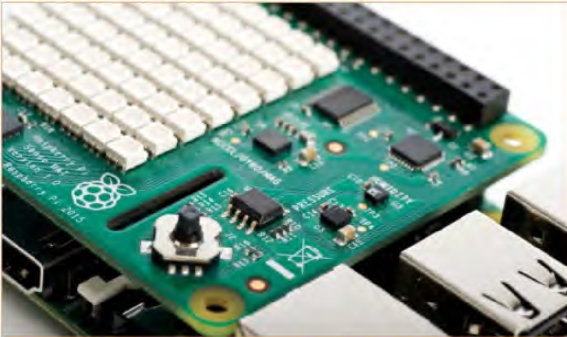
Left We'll use the tiny joystick in the bottom-right corner as the input for our selection interface
