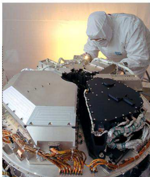
THE INFRARED ARRAY CAMERA (IRAC) aboard the Spitzer Space Telescope takes images covering a 26-square-arcminute area, or, for comparison, about 3 percent of the area of the Full Moon. IRAC images in four infrared channels simultaneously. The channels' wavelengths center on 3.6, 4.5, 5.8, and 8 micrometers. IRAC's only moving part is its shutter. NASA/JPL-Caltech
