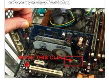
Take your new card, holding it so that you don't damage any of the components or touch the contacts tab and position in over the same PCIE slot from which you just removed your old card.
