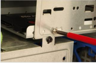
Step 14 If you've already installed your SSD, open up the PC case again and disconnect the old hard drive. If you don't plan on using the HHD again you can remove it. You'll need a small cross-head screwdriver to undo the screws holding the drive into the bay.
