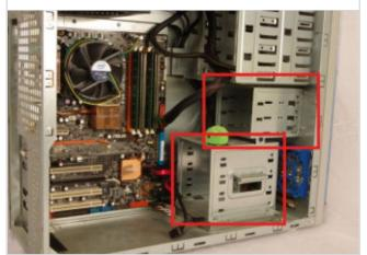
Your new SSD should come with an adapter plate to fit it into a 5.25-inch drive bay, as well as the required fitting screws. The first action is to attach the SSD to this plate. Don't over-tighten the screws or you may damage the drive.
