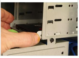
Step 7 Using the supplied mounting screws, fix the mounting plate holding the SSD in position. If you can't easily access all four screw holes don't worry; as long as the drive doesn't move just using two screws will be fine.
