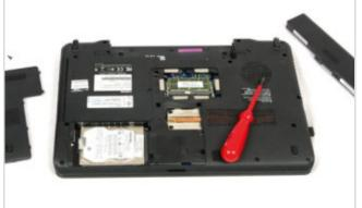
Step 14 Before touching any internal components, earth yourself by briefly touching a radiator water pipe to dissipate any static charge in your body.
