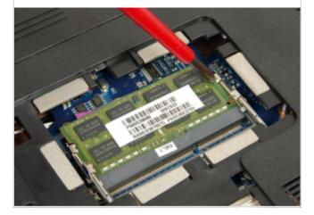
Carefully and gently pull out the old memory modules, noting the orientation and the position of the gap in the contacts tab. If it won't move, check that you've fully released the clips. Don't force it!
