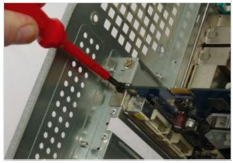
Step 8 Carefully ease the card out of the motherboard slot.
