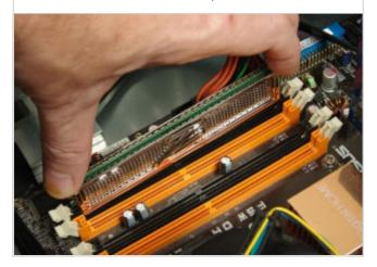
Step 11 Gently push the new module down into the slot. You'll see that the plastic retaining clips partially close as you do so. When the module is all the way in, close the retaining clips to lock it in place.
