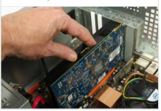
Refit the screw or clip that secures the card to the back of the PC case, where the monitor cable goes.
