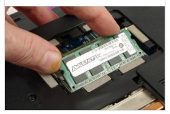
Once the module is seated in the slot, push it back down flat until the sprung clips snap into place.
