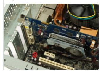
Once the uninstallation process is complete, shut down your computer, unplug the mains lead, disconnect the mouse, keyboard, monitor and any other attached devices, then leave it for half an hour to ensure that residual voltage in any capacitors has dissipated and any hot components have cooled down.
