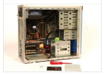
Step 3 AN SSD can fit into either a 3.5-inch (floppy disk drive) bay or a 5.25-inch (HDD/optical drive) bay. Since many recent PC cases no longer have 3.5-inch bays we'll show how to fit your SSD into the larger 5.25-inch bay.
