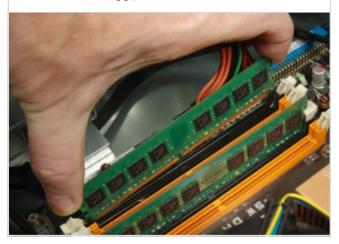
Taking care not to touch the metal contacts, carefully position your new RAM modules in the slot, making sure to line up the slot in the contact tab with the gap in the modules slot, the same as the module you removed.
