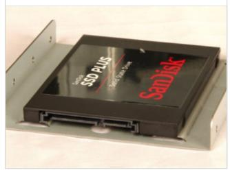
Once you've decided on a good position for the SSD within the drive bay, carefully slot the drive on its mounting plate into the drive bay. Position it so that the screw holes on the PC chassis line up with the holes on the mounting plate.
