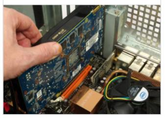
Carefully push the card down into the slot. If it won't go all the way in, check for obstructions such as stray cables. Don't force it or you may damage both the card and your motherboard. You should hear the click of the retaining catch when it's all the way in.
