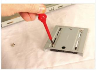
Step 5 Note that one end of the SSD has the connectors on it.
