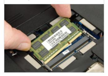
Taking care not to touch the metal contacts, carefully position your new RAM module in the slot, making sure to line up the slot in the contact tab with the gap in the module slot, the same as the module you removed. Gently push it into the slot.
