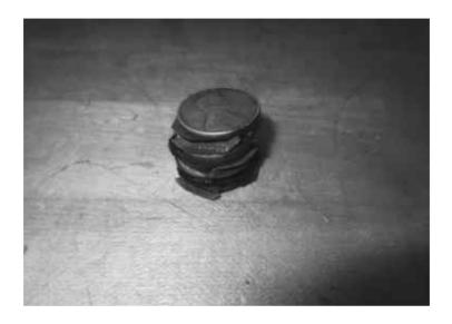
**Step 10:** Wrap a piece of electrical tape around the battery to hold it together.
