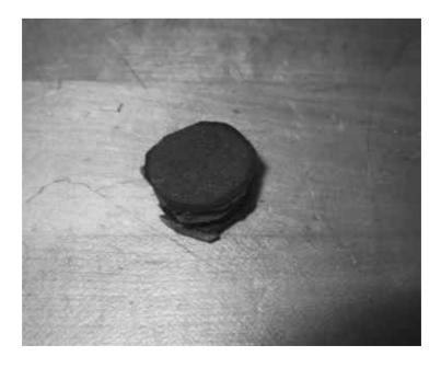
**Step 9:** Put another penny on top and repeat the pattern again. From top to bottom, you should have: washer, disk, penny, washer, disk, penny, washer, disk, penny. This creates a battery with three cells, which will be enough to light an LED bulb.
