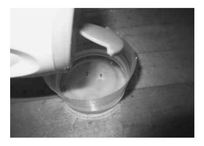
**Step 4:** Stand the 9-volt battery up on the kitchen counter. Lower the plastic cup of water until both battery terminals touch the heads of the thumbtacks.
