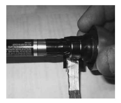
**Step 6:** Attach the other strip to the end of the batteries securely with electrical tape. Use the piece of tape across the end of the battery and pull it tight. You can test your connection by touching the two aluminum strips together. The light should come on if your connections are tight. Repair any connections if the light doesn't come on.
