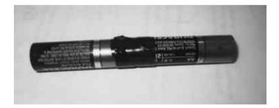
**Step 3:** Hold the head assembly and the batteries together and use another 4-inch strip of electrical tape to keep them together. The head assembly and the batteries should be tight and stay together. Retape if they aren't tight.
